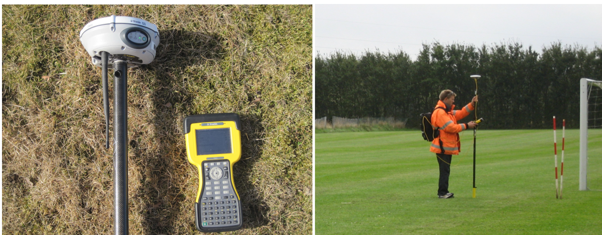
Figure 3.1: Measuring with RTK-GPS equipment
