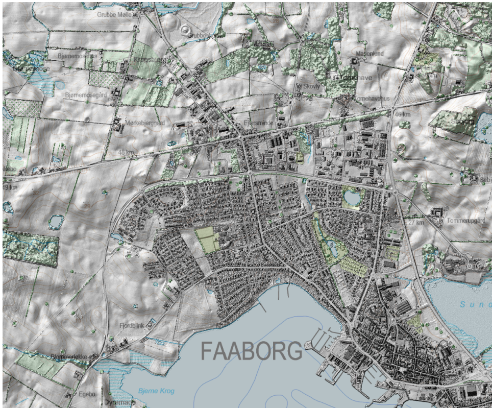
Figure 1.2: Visualization of DK-DEM/surface in combination with a topographic map.
