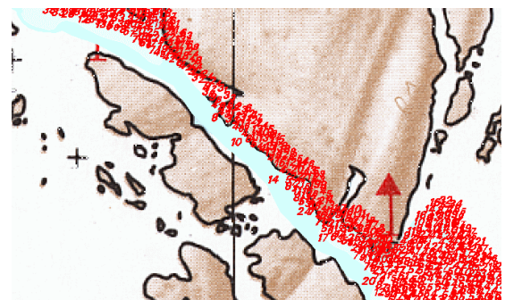
Figure 3: Differences between the old chart no. 1212 and a set of newly measured multibeam data (shown in red). It is evident that the coastline registrations need adjustment.
