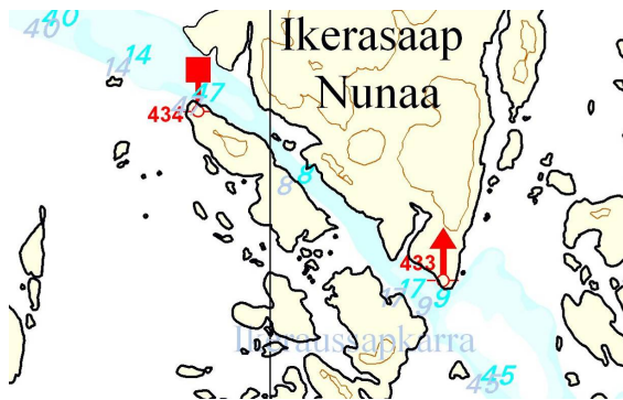
Figure 9: Effects of the transformation of existing soundings: old positions printed in grey, new in cyan.
