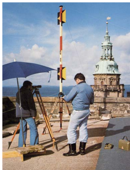
figure 5: Optical water crossing from the top of Telegraph Tower aiming to the signal plates in Sweden
