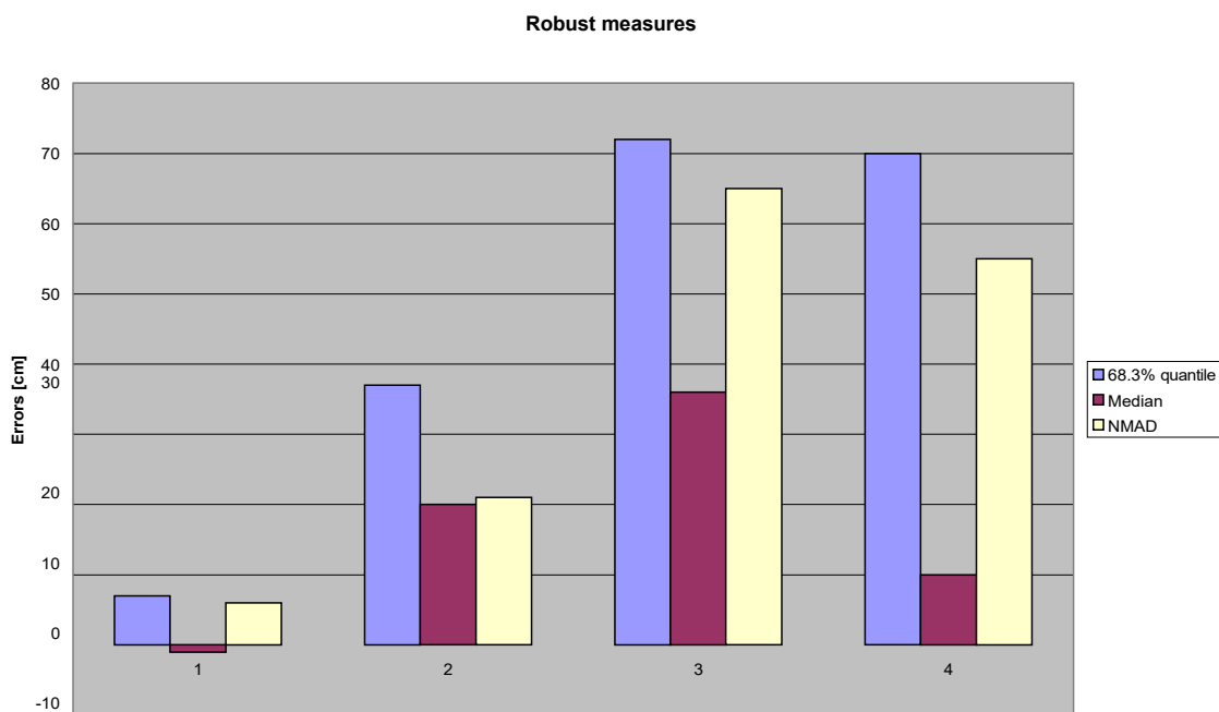
Figure 10. Results of test with 10 cm images (test A), robust measures. It means 1: Laser/GPS, n= 257, N=6; 2: foto_filtr/GPS_GCP (n=13, N=0); 3: foto_filtr//GPS/CP (n=231, N=3); 4: foto_filtr/Laser (n=259446, N=5734)
