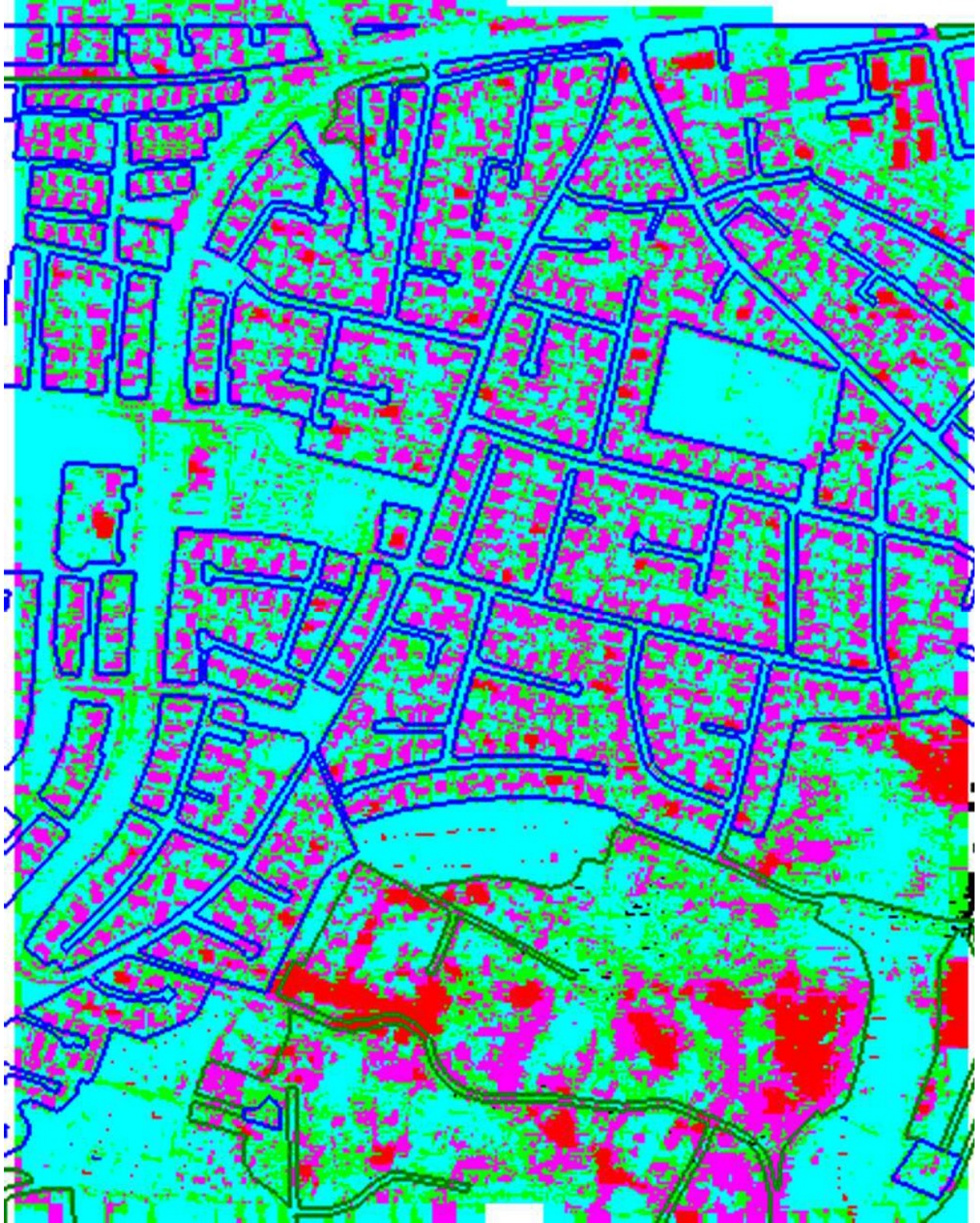
Figure 12 : Result of filtering of the photogrammetrically derived DSM using the strategy “hoe1”. The classes are buildings (red colour), forested area (green colour) and gross errors (violet colour). The non-classified areas are the “open areas” depicted in blue colour.
