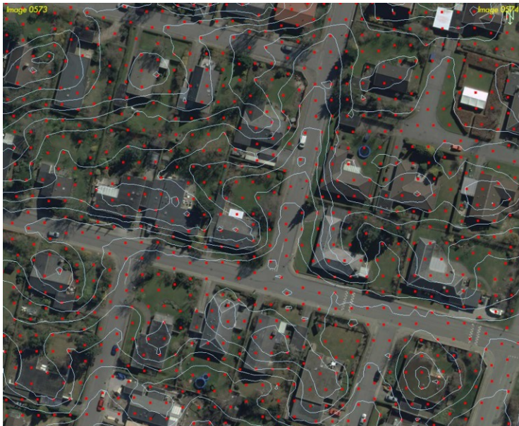
Figure 26. Aerial image together with elevation dots and contour lines. Monoscopic editing is usable for some of the editing functions only.
