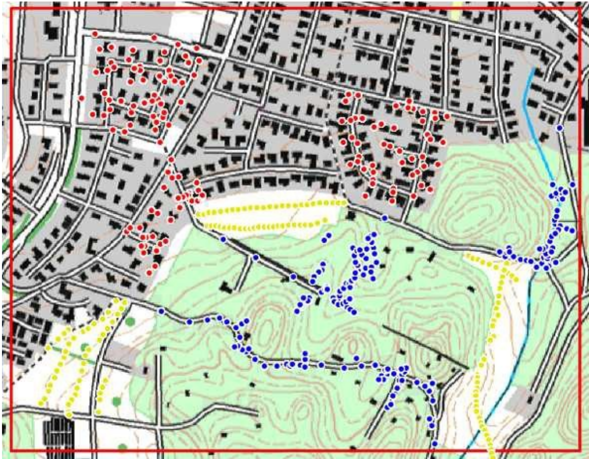
Figure 2. Distribution of checkpoints. The checkpoints are plotted in yellow colour for open terrain, in red colour for the built-up area and in blue for the forested area.
