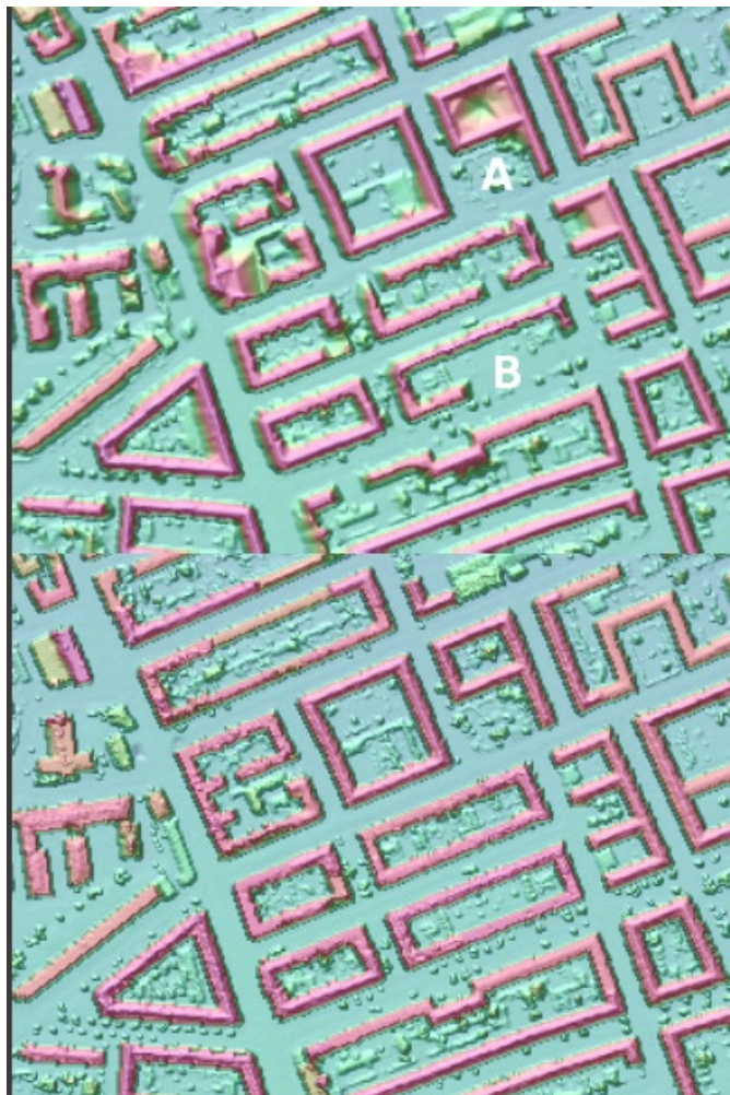
Figure 1: City DSM before (upper panel) and after (lower panel) incorporation of a priori data from a land use/land cover (LULC) model. Note how the backyard vegetation giving problems (near A) are fully resolved after incorporation of LULC. Also, the missing building (near B) is reconstructed by validating the few reflections actually available against LULC information that a building really is expected here.
