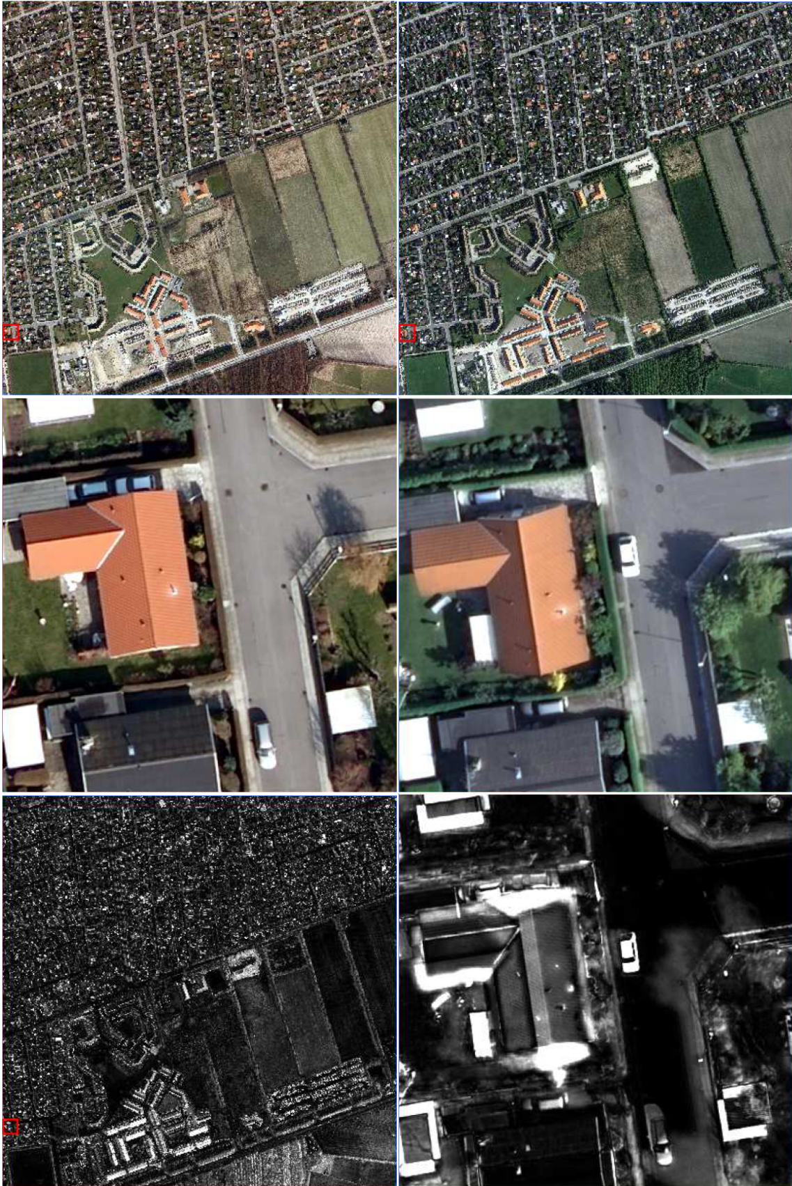
Figure 12: Example of registration problems. Changes between years 2007 and 2008. UL: The 2007 scene. UR: The 2008 scene. ML: Zoomed area from the 2007 scene. MR: Zoomed area from the 2008 scene. LL: Full scene change image. LR: Zoomed area change image.
