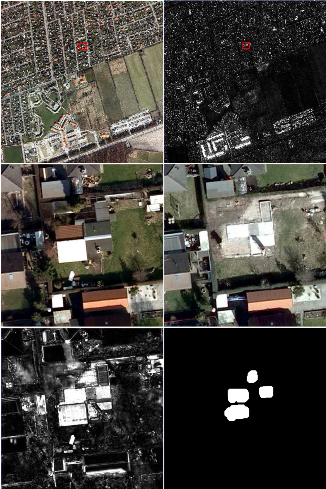
Figure 5: Example 3 for area from 6168_726. Changes between years 2007 and 2009. UL: The 2007 scene. UR: Change image. ML: Zoomed area from the 2007 scene. MR: Zoomed area from the 2009 scene. LL: Change image. LR: Significant change image.
