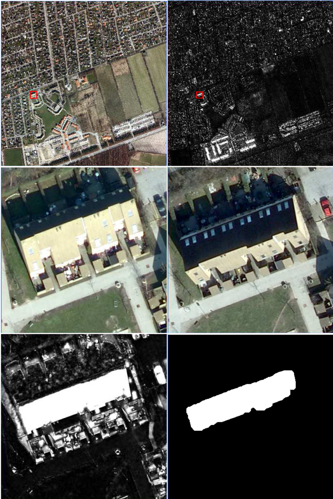
Figure 11: Example 9 for area from 6168_726. Changes between years 2007 and 2009. UL: The 2007 scene. UR: Change image. ML: Zoomed area from the 2007 scene. MR: Zoomed area from the 2009 scene. LL: Change image. LR: Significant change image.
