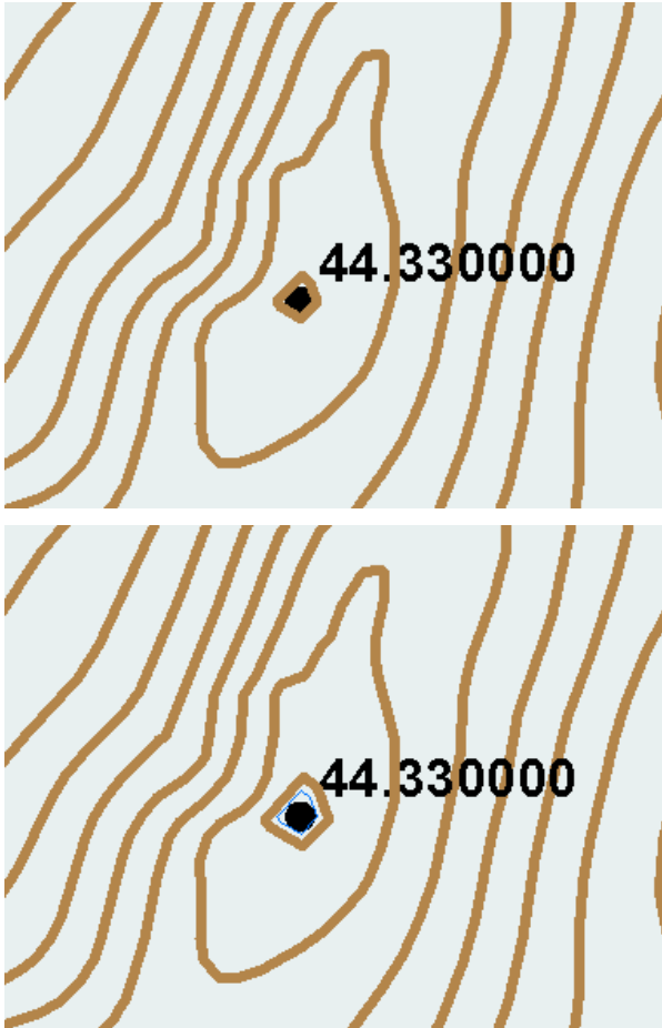
Figure 6: The curve around the height point has been extended, so that the symbol for elevation points becomes visible.
