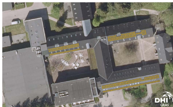
Deep learning approach to automatically segment solar cells on rooftops from very high-resolution satellite imagery.
