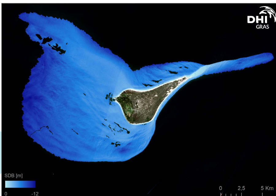
Satellite-derived bathymetry for the area surrounding Anholt produced to supplement a multibeam survey.
