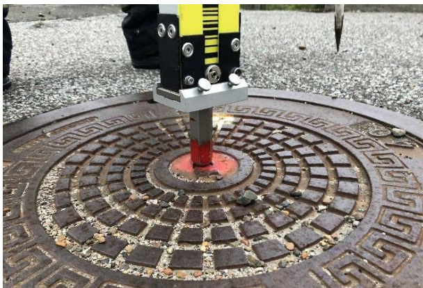
Figure 1. Surveyor stage with adapter placed in the middle of the manhole cover defined as the “measuring point” on all covers.
