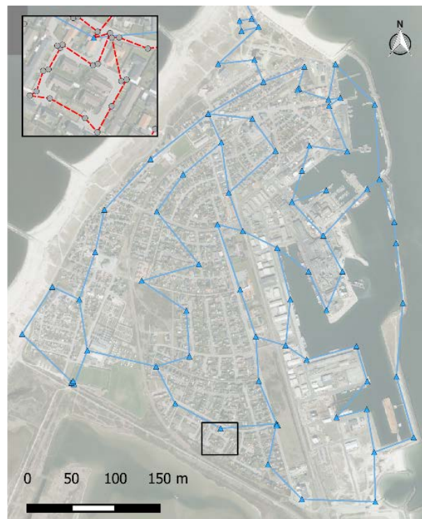
Figure 2. The benchmark measuring campaign in Thyborøn showing how the levelling to each manhole cover is tied to the benchmark network.
