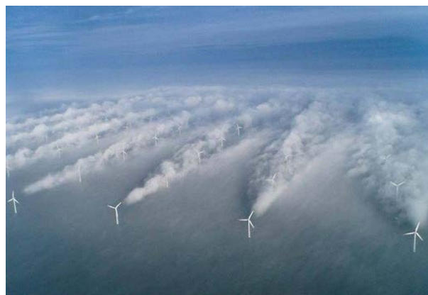
Wind farm wake at Horns Rev 1 offshore wind farm in the Danish North Sea. Source: Vattenfall.
